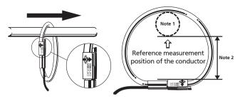
Note 1: Reference measurement position of the conductor. Maximum coupling diameter: 20 mm for published accuracy.
