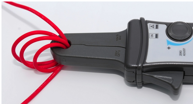
Figure 7: Increasing the sensitivity
