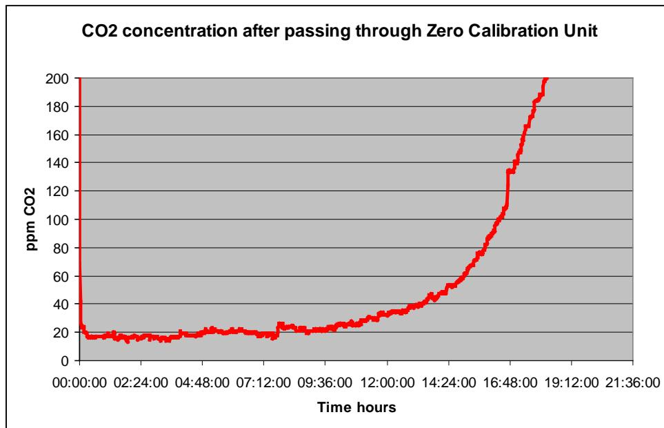
For best result the Zero Calibration Kit should be in operation a while after changing the CO<sub>2</sub> absorbent cartridge so that the cartridge will stabilise.
