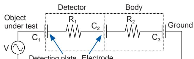
Although a detected current will flow to the ground through your body, the current, less than 1  $\mu$ A, will not adversely affect you.
