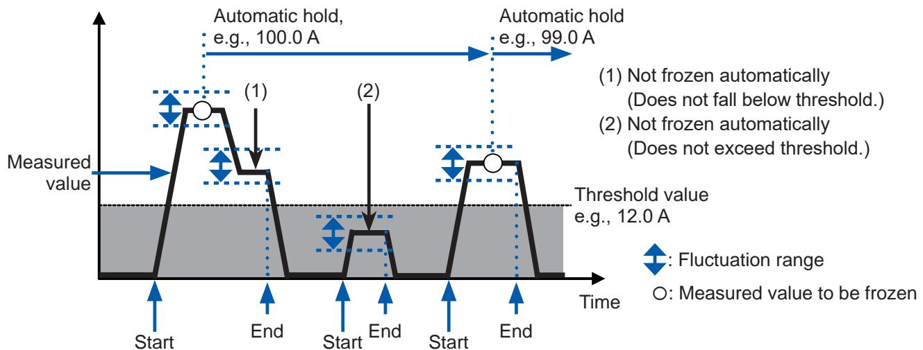
Suppose that the measured value has fallen below (voltage, current) or exceeded the threshold value (resistance, continuity, diode) after the displayed value froze. When the two auto-hold conditions are met again after that, refreshing measured values will stop.
