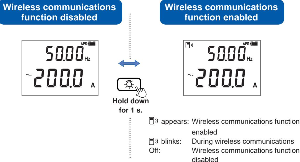
When the instrument is turned on for the first time after the Z3210 has been installed, the wireless communications function will be enabled.
