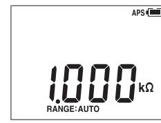
If resistance values of coils, including motors and transformers, measured with the auto-ranging fluctuate, select the range manually.
