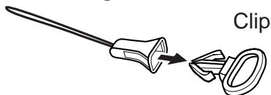
**3** Attach the strap buckle to the instrument and connect it to the clip that you attached to the P2000 with the strap.
