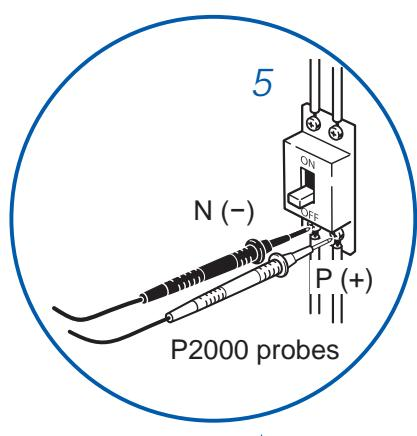
5 Bring the probes into contact with an object to be measured.
