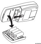
Remove the yellow boot to access battery door. 4 AA batteries (alkaline recommended) 20 hours typical battery life.
