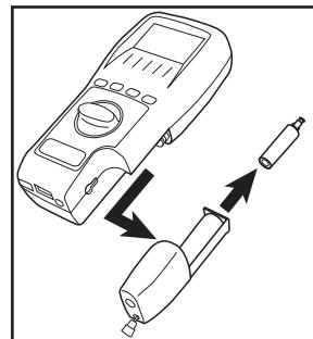
Remove the probe from the flue and allow the analyzer to purge with fresh air until readings return to zero. - O2 to 20.9%, CO to Zero (Be careful as the probe tip will be HOT)
