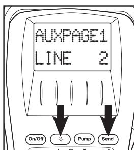
AUXPAGE1 LINE 2 shows press "Send" to continue to set line 2. Press "▲" UP or "▼" DOWN select between available parameters and press ENTER "⬅" to set.
