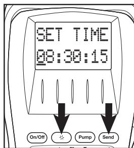
Clock displays with the cursor underneath the first digit. Press "▲" UP or "▼" DOWN to increase or decrease and press
