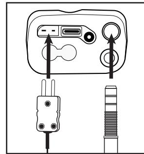
NOTE: Take care when inserting the temperature probes as the pins are polarized. Insert with the smaller pin (+) to the right.
