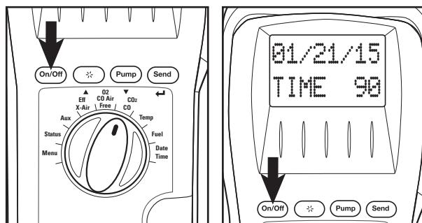
Power on in area of fresh air and allow to countdown. On sealed combustion appliances (ducted inlet) connect flue probe and power on outside and allow to countdown to set inlet temperature. (see page 12)
