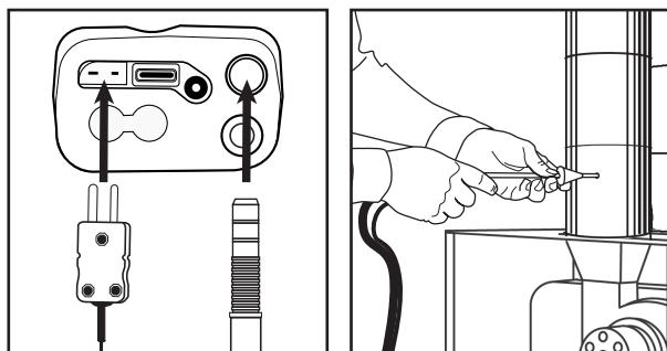
Connect flue probe thermocouple connector to T1, and connect flue probe to water trap as shown above.
