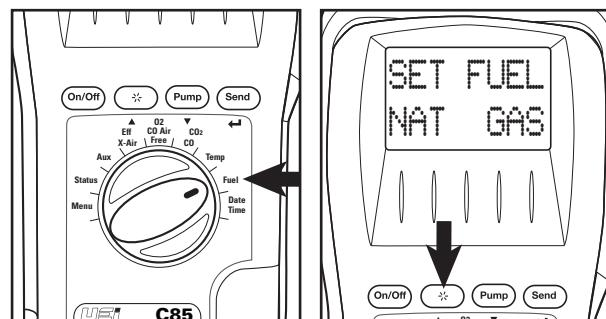
Rotate test selector to **Fuel**.
