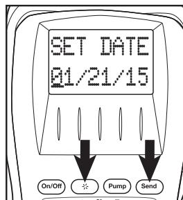
Date displays with the cursor underneath the first digit. Press "▲" UP or "▼" DOWN to increase or decrease and press
