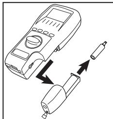
This is a very important part of the analyzer and should be changed regularly. It prevents dust and dirt particles from entering the pump and sensors that will cause damage. The filter **MUST** be changed when it appears discolored on the inner surface.
