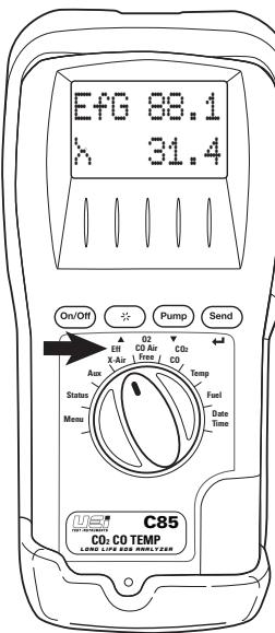
Rotate selector to **Eff X-Air**. The Eff/X-Air screen shows calculated combustion efficiency using a Gross Condensing calculation and excess air. When below condensing temperature the efficiency calculation includes and estimated energy recovered during condensation that increases combustion efficiency.
