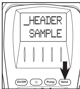
The existing HEADER 1 will display with the cursor underneath the first digit.
