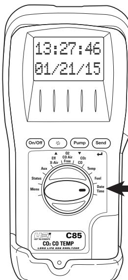
Rotate test selector to **Date Time**.
