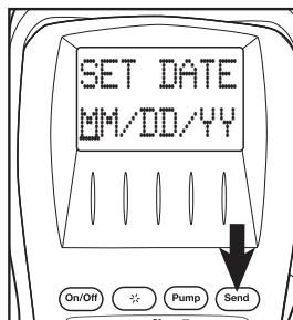
Set date displays with MM/DD/YY Press "▲" UP or "▼" DOWN to select a different format press
