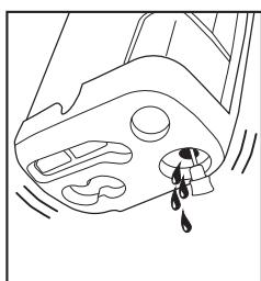
The in-line water trap should be checked and emptied on a regular basis. Water vapor will condense in the probe line, which may cause the water trap to fill suddenly if the probe is moved. Care should be taken at all times.
