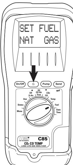
Rotate test selector to **Fuel**.
