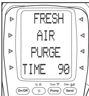
Power on in area of fresh air and allow to countdown. On sealed combustion appliances (ducted inlet) connect flue probe and power on outside and allow to countdown to set inlet temperature. (see page 12) Note: Not required if using inlet probe in T2.
