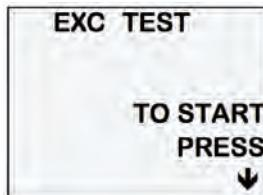
The C165 will wait 60 seconds and then record the Post-Blower values for CO, O<sub>2</sub> and Excess Air.
