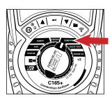
Rotate the selector dial to PRS/TEMP
