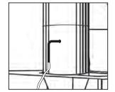
Place combustion probe or true draft probe tip in the flue to measure draft.
