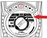
Rotate dial to EXCH TEST. Press **t**o start.
