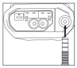
Insert Flue probe into stack. Adjust cone so end of the probe is approximately at the center of the stack.
