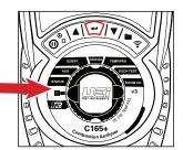
The **AUX** screen allows you to assign any of the following parameters on any display line. CO<sub>2</sub>, CO, NO (if fitted), NO<sub>x</sub> (if fitted), O2, TF, Ti, Ta, Delta (Δ), Loss, EFg, Xair, Ra (CO/ CO<sub>2</sub> Ratio), PI, Fuel Type, PRS or Blank.
