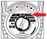
Rotate the selector dial to PRS/TEMP.
