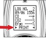
To print the LOG, Press and very buttons until PRINT is selected between two arrow icons. Press 🕶 to select to start printing.
