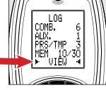
Screen displays all saved LOGS. With VIEW selected in the Status Bar, Press to select.
