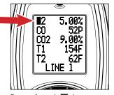
Press ▲ and ▼ buttons to scroll parameter selections. Press to select a parameter and advance to the next Line.
