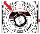
Rotate the dial to either AUX, 02/Eff, C0/C02 or TEMP setting.
