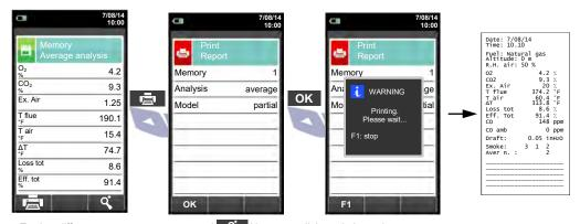
To view different test measurements, use ' ' key to scroll through the various test measurement screens. **Tg** = Flue Gas Stack Temperature **Ta** = Ambient or Incoming Air Temperature Xair = Excess Air AT = Differential Temperature (NET Temperature) Eff. tot = Total Combustion Efficiency Loss tot = Stack Losses
