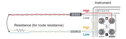
At this time, use the assembled calibration cable for a terminal to be calibrated (in the figure, Source Hi).
