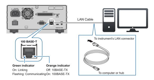
If the green indicator fails to light up after connecting the instrument to the LAN, there may be a malfunction in the instrument or connected devices, or the LAN cable may have a break or a poor contact.
