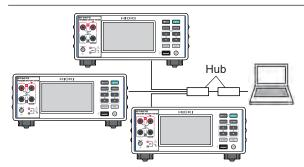
In addition, after creating a program, connecting external equipment, such as a computer to the communications command port using TCP allows you to control the instruments through communications commands. See Communications Command Instruction Manual for details.
