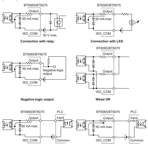
Connection with PLC input (positive-common) Connection with PLC input (negative-common)
