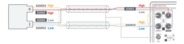
Use four terminals to make measurement. When making measurements with two terminals (using 4-into-2 interconnected wire pairs), measured resistance values may vary due to various factors, including effect from wire resistance and contact resistance\*1 in the test-lead assembly. Additionally the instrument may display different readings each time with each measurement.
