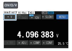
Press the  $\Omega V/\Omega/V$  key to select the resistance/voltage measuring function ( $[\Omega V]$ ) or voltage measuring function ([V]).
