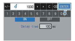
4 Use the numerical keypad to enter the trigger delay time.
