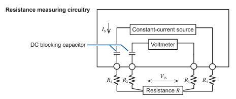
R<sub>1</sub> to R<sub>4</sub>: Resistance of the test-lead wires and contact resistance of contact points
