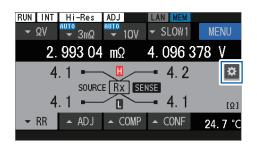
While making measurement with the resistance measuring function ( $[\Omega V]$  or  $[\Omega]$ ), tap [RR] or press the DISPLAY key.
