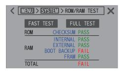
Once the test is completed, the test result is displayed.
