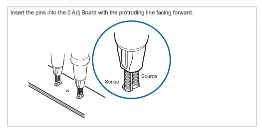
The pin-supporting part has a protruding line on the Sense side. Face these lines in the same direction when performing zero adjustments. Select two holes on the 0 Adj Board arranged symmetrically with respect to the line through the center plus sign, ensuring they are positioned at approximately the same distance as the terminals of the battery under measurement, then press the pins against the bottom of the holes.
