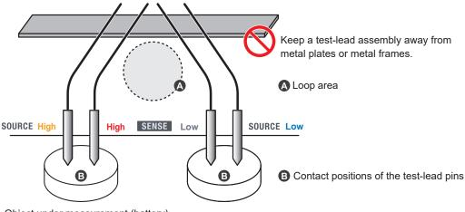
Object under measurement (battery)
