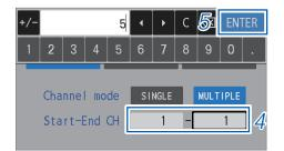
Use the numerical keypad to enter the start and end channels for the referential adjustment.
