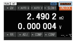
During key lock activation, [KEYLOCK] is displayed in the top right corner of the screen.
