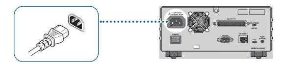
If power is interrupted, such as by a circuit breaker tripping, while the Power switch is set to the on position, the instrument will automatically turn on once power is restored.
