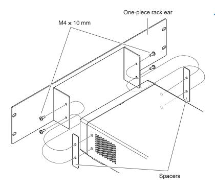
Insert the spacers between the rackmounting ear(s) and both sides of the instrument and attach the ear(s) with the specified screws (four in total).
