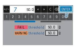
Use the numerical keypad to enter the warning threshold.
