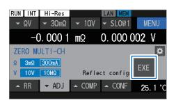
If the presently set measuring function or range differs from when the adjustment values are obtained, the values are not applied. The adjustment setting screen is displayed as illustrated on the left.
