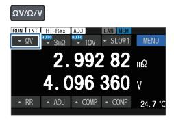
Press the  $\Omega V/\Omega/V$  key to select the resistance/voltage measuring function ([ΩV]) or resistance measuring function ([Ω]).
