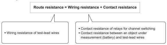
The route resistance is measured simultaneously with the internal resistance of a battery. Continuous monitoring of the route resistance allows effective maintenance management of a measurement system. Additionally, thresholds can be defined for route resistance measurement, enabling a three-level judgment (Pass, Warning, and Fail).
