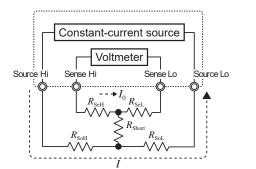
$$\begin{split} E &= (I_0 \times R_{\text{SeL}}) + (I_0 \times R_{\text{SeH}}) \\ \text{When } I_0 &\approx 0 \\ E &= (0 \times R_{\text{SeL}}) + (0 \times R_{\text{SeH}}) \\ &= 0 \text{ [V]} \end{split}$$
