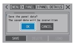
${\it 3}$  To overwrite the existing measurement conditions with the present ones, tap [OK].
