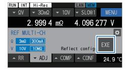
If the presently set measuring function or range differs from when the adjustment values are obtained, the values are not applied. The adjustment setting screen is displayed as illustrated on the left.
