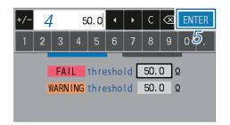
4 Use the numerical keypad to enter the fail threshold.
