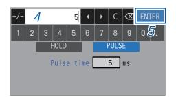
4 Use the numerical keypad to enter the pulse width.
