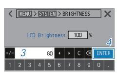
Use the numerical keypad to enter the backlight-brightness level.
