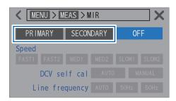
Use the primary instrument to tap [PRIMARY]. Use the secondary instrument to tap
