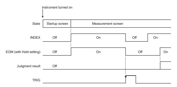
Judgment results: R\_HI, R\_IN, R\_LO, V\_HI, V\_IN, V\_LO, R\_R\_PASS, R\_R\_WARNING, R\_R\_FAIL, PASS1, FAIL1, PASS2, and FAIL2, including ERR This timing cart indicates the operation when the trigger source is set to external.
