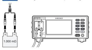
Obtaining adjustment values for each channel (position)
