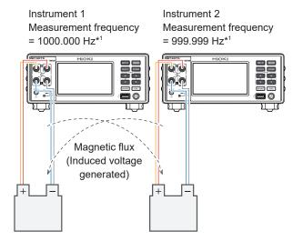
Simultaneous measurement can result in mutual interference due to electromagnetic induction.
