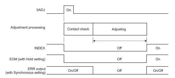
The ERR signal turns off upon successful zero adjustment and turns on if the adjustment fails. If the 0ADJ signal is input during a measurement, the instrument suspends the measurement, starting single-mode zero-adjustment.
