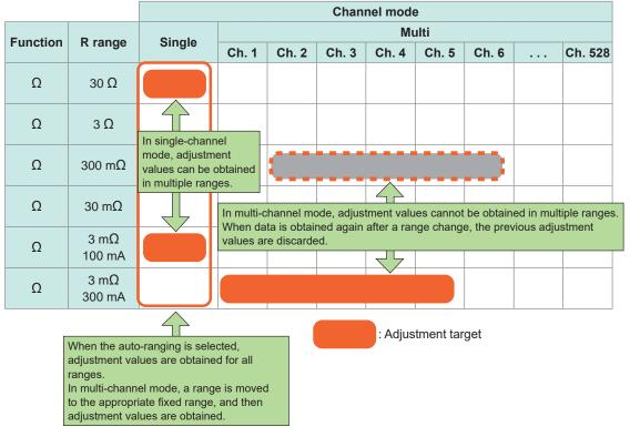
The measurement accuracy of resistance and DC voltage is specified on the condition that the zero-adjustment is completed.
