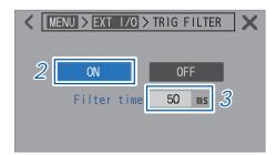
Tap [ON] to turn the filter capability on.
