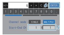
Use the numerical keypad to set the channels that start and end the zero adjustment.
