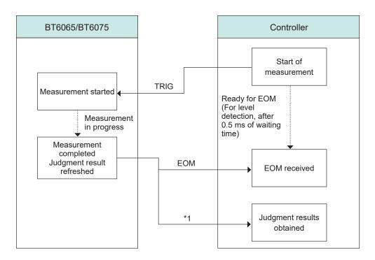
\* 1. R\_HI, R\_IN, R\_LO, V\_HI, V\_IN, V\_LO, R\_R\_PASS, R\_R\_WARNING, R\_R\_FAIL, PASS1, FAIL1, PASS2, FAIL2, and ERR
