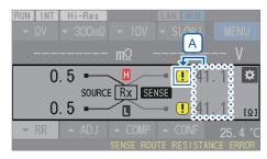
• B The route resistance of the Source Hi terminal exceeds the display range.
