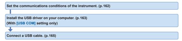
Before connecting the instrument to a computer, download a USB driver to install.
