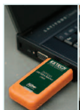
BRD10 - Optional Wireless USB Video Receiver allows user to stream live video to a PC and also can be remotely viewed via VOIP connection
