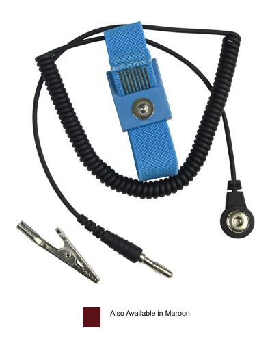
This standard performance wrist strap set features a fully adjustable stretch fabric wristband and coil cord. The wristband provides a 360 degree conductivity around the wrist for maximum skin contact. Wristband curling is reduced by the woven wristband fabric. This wrist strap features an adjustable fabric wristband with a 6-foot retractable coil cord, alligator clip and a 4mm snap. Wristband available in blue or maroon. Meets ANSI/ESD S20.20 and ANSI/ESD S1.1.
