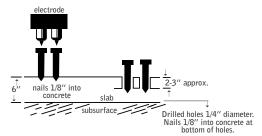
If the meter still indicates green or "dry," the floor should be ready for covering. Tests should only be made in newly drilled holes, since the inside surface of the holes can dry out while the rest of the slab is still wet.
