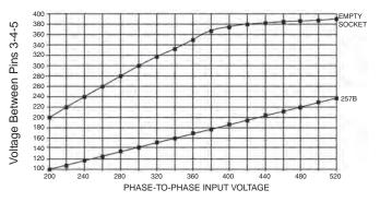
As shown above, with a monitor inserted in the socket, the voltage on pins 3, 4, and 5 (inputs to the monitor) is limited to the operating range of the monitor. The voltage change is linear over the full adjustment range of the monitor. With the monitor removed (and power applied) the voltage potential rises to the input voltage level. However, from approximately 380Vac to 520Vac the Smart Socket limits the voltage potential so that it never rises above 395Vac.
