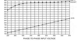
As shown above, with a monitor inserted in the socket, the voltage on pins 3, 4, and 5 (inputs to the monitor) is limited to the operating range of the monitor. The voltage change is linear over the full adjustment range of the monitor. With the monitor removed (and power applied) the voltage potential rises to the input voltage level. However, at approximately 380Vac to 635Vac the Smart Socket limits the voltage potential so that it never rises above 390Vac.
