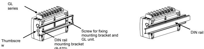
GL series can be mounted to DIN rail using mounting bracket B-570. The mounting bracket is fixed to rail by thumbscrew.
