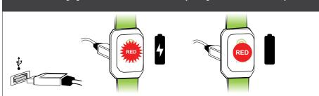
Aura can be used up to 12 hours on a single charge. When battery is low the LED will flash red and device will vibrate every 1 minute.
