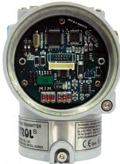
Figure 6-3 Structure of Electronics Module inner Transmitter
