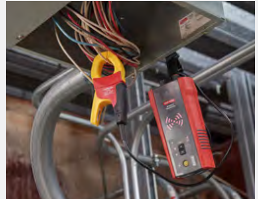
Intuitive transmitter automatically senses whether the system is energized or de-energized
