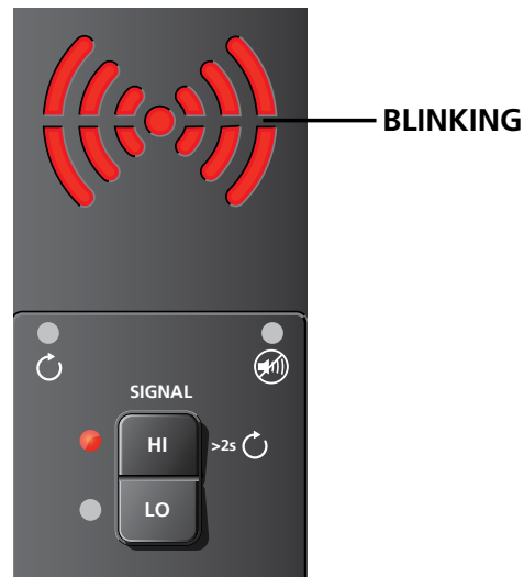
Figure 3.1b: Transmitter indicator showing signal in HIGH mode
