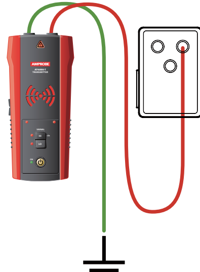
Figure 3.2b: Separate ground connection (Preferred)
