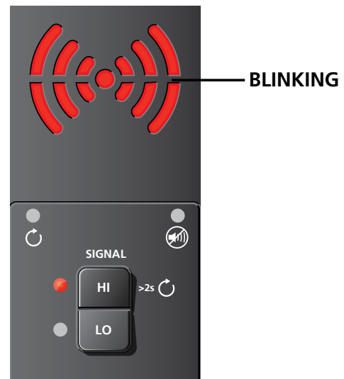
Figure 4.12b: Transmitter indicator showing signal in Loop mode
