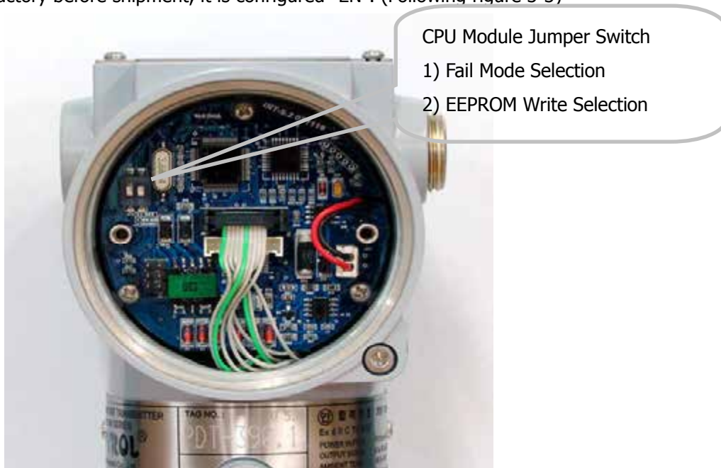
Figure 3-3. CPU Module Fail Mode, EEPROM-Write Selection Jumper Switch
