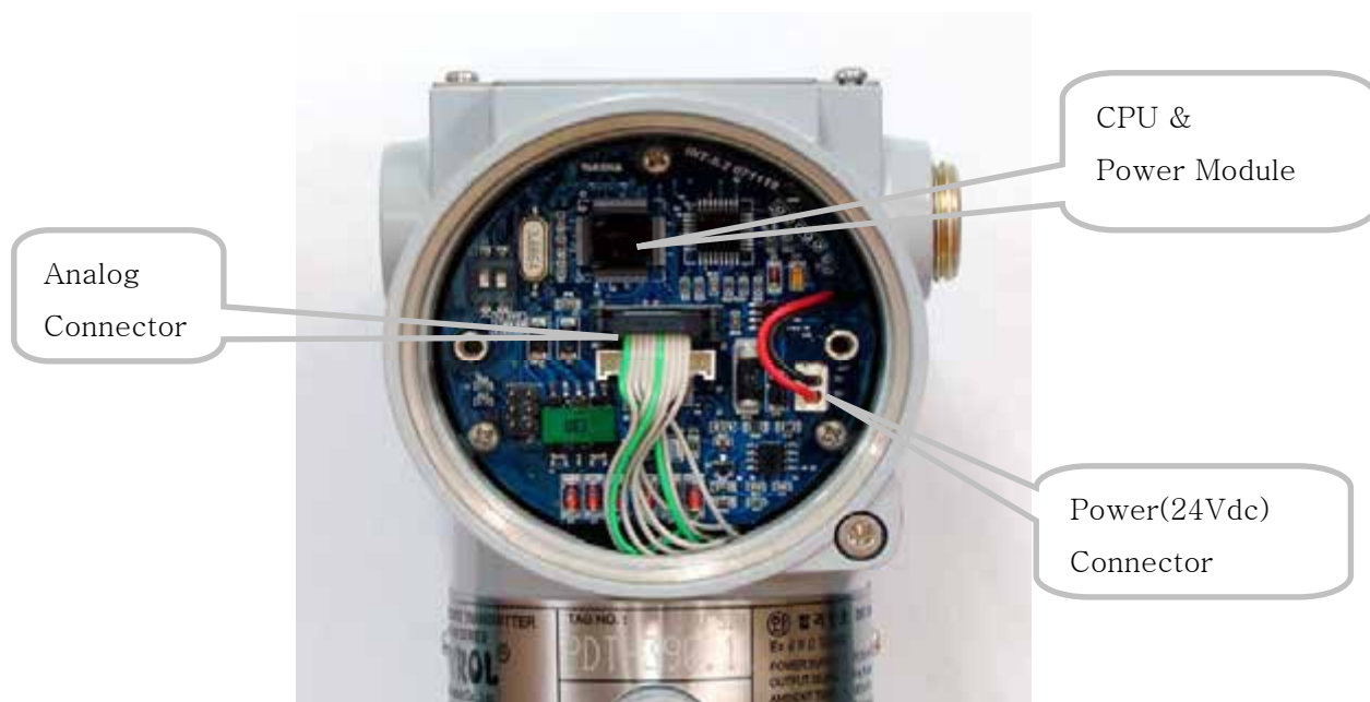
Figure 6.3 Structure of Electronics Module inner Transmitter
