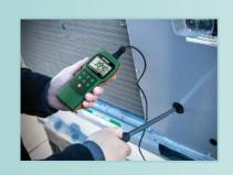
Telescoping probe with 18mm diameter vane sensor easily fits into air vents and can extend length of probe to 3.3ft (1m) long. Measures Air Velocity/Volume, Temperature, Humidity, Wet Bulb, and Dew Point. User can store up to 12,000 readings for data analysis.
