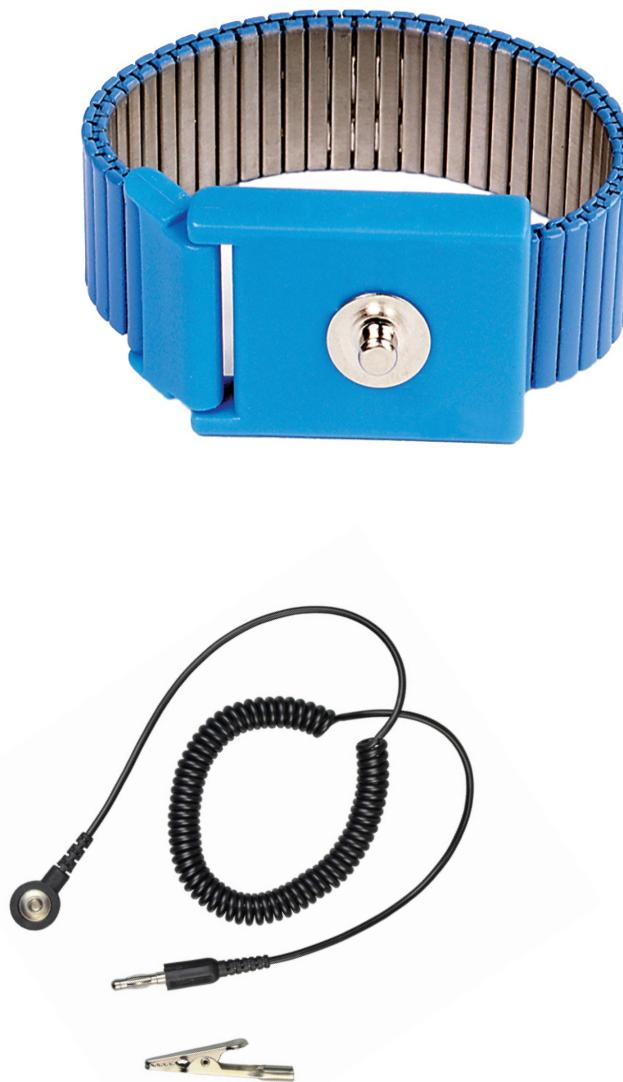
Made from stainless steel, the durable premium performance metal wristband creates a reliable electrical contact to the user's wrist. The flex-metal style band uses adjustable links to assure a secure and comfortable fit. The retractable coil cord terminated with a banana plug on one end and connects to the wristband via a 4mm post snap and contains a 1 megohm resistor. Includes alligator clip. 6 or 12 foot cord length is available.
