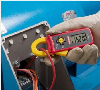
**Utilize the inrush current** function for motor start-up monitoring.
