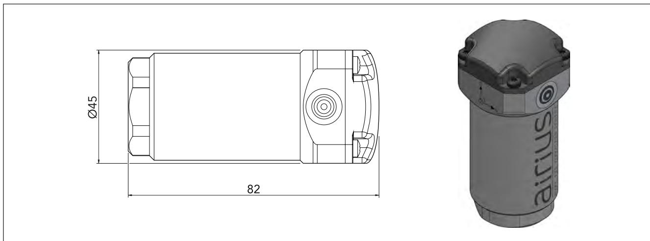
Airius is a wireless, battery-powered sensor that performs a user-defined number of vibration measurements per day in the 10-1000 Hz or the 2-1000/10-5000 Hz frequency range. The MEMS (micro-electro-mechanical-systems) type sensor with digital output measures triaxial vibration and temperature.
