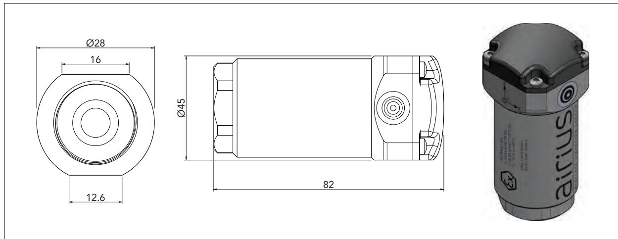
Airius is a wireless, battery-powered sensor designed for vibration monitoring of industrial machines in areas with potentially explosive atmosphere. It performs a user-defined number of vibration measurements per day in the 10-1000 Hz or the 2-1000/10-5000 Hz frequency range. The MEMS (micro-electro-mechanical-systems) type sensor with digital output measures triaxial vibration and temperature.
