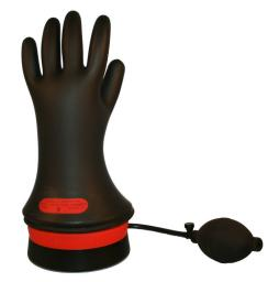
The IGO-11-9 (Class 0, 11" length glove, size 9) with the Cementex glove inflator (CPGI), which enables thorough visual inspections which are required prior to each use.
