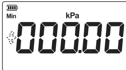
Figure 14 Lower limit calibration point
