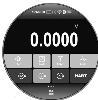
Figure 6 Electrical signal measurement function
