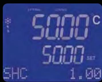
For further optimization of temperature control, you can easily input the specific heat capacity value for the heat transfer fluid that you're using.
