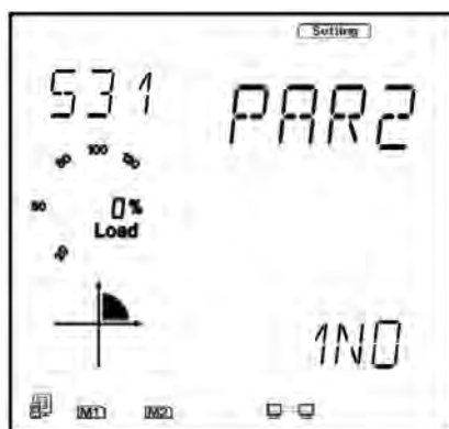
Figure 5-54 Parity setting for the AXM-RS485 module
