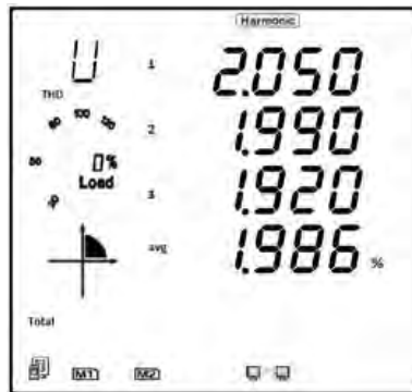
Figure 3-21 - Harmonic Distortion Reading
