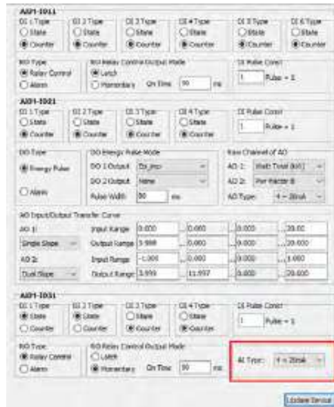
Figure 5-45 Analog Input Type Setting
