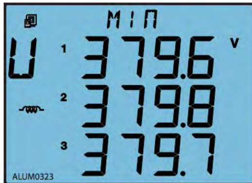
Fig.3-25 Min value of phase voltage
