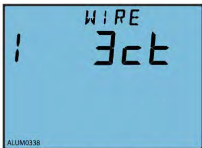
Fig.3-41 Current input wiring setting
