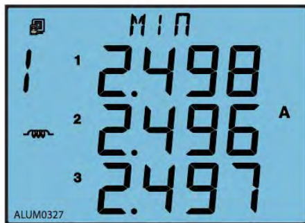
Fig.3-29 Min value of current
