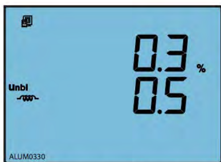
Fig.3-32 Unbalance factor for voltage and current
