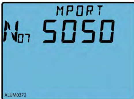
Fig.3-79 MODBUS-TCP port setting
