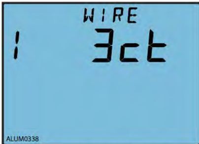
Fig.3-41 Current input wiring setting
