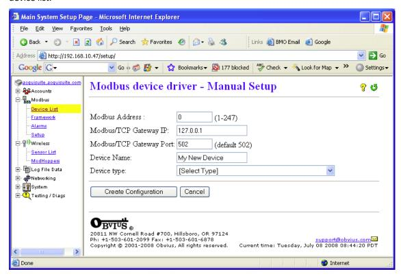
The manual setup page has several options that must be configured before the EMH+ will recognize the Modbus device. The options are as follows:
