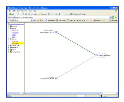
The graph will draw a blue box for each ModHopper that is attached to the system. The blue number inside the box icon is the Modbus address of the ModHopper. To the side of each icon, three lines of information will be shown.
