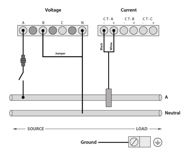
Note: The jumper wire between B and N in this configuration must be the same wire size as the Neutral wire.
