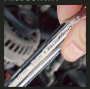
Serrated wrench beam allows you to feel which direction to pull.
