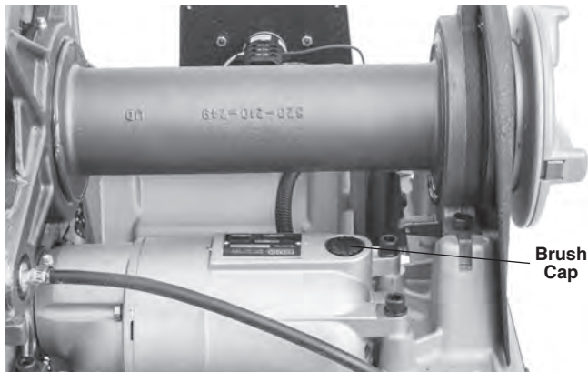
Figure 34 – Removing Motor Cover/Changing Brushes
