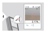
Aim laser at upper points and angle/height tracking starts automatically.
