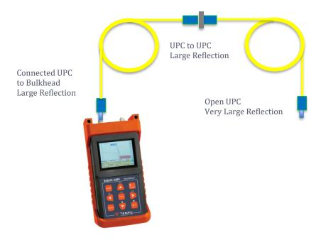
Mated UPC connections have high reflectivity (~45dB) An open (not connected) UPC will have a very high reflectivity (~14dB)
