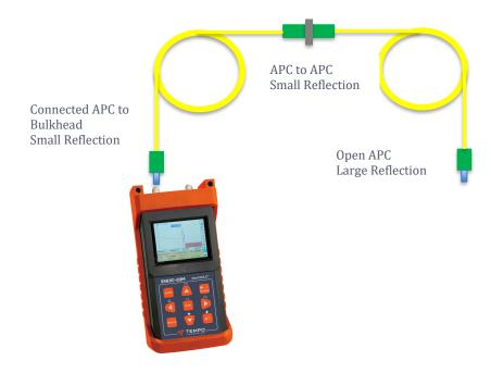
Mated APC connections have very low reflectivity (<65dB typical) An open (not connected) APC will have a high reflectivity (~45dB)
