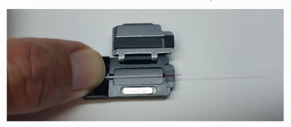
The 900 micron loose tube must not be held by the small fiber clamp on the far right hand side but only with the larger main clamp.
