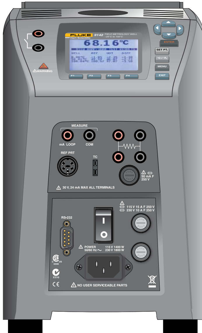
Figure 2 914X Field Metrology Well
