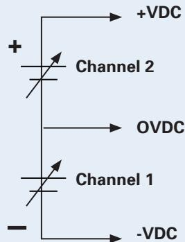
This feature is useful for powering bipolar circuits and devices.
