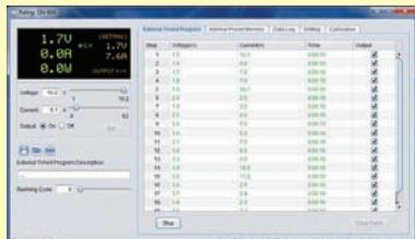
Control your instrument through remote control PC software or use programming commands to communicate with your instrument.
