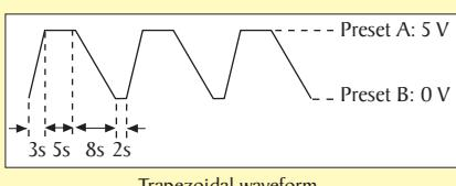
Use the front panel preset buttons to quickly set and recall up to 3 different voltage and current settings, to program the power supply for transient mode operation and to output bi-level square, triangular or trapezoidal waveforms.
