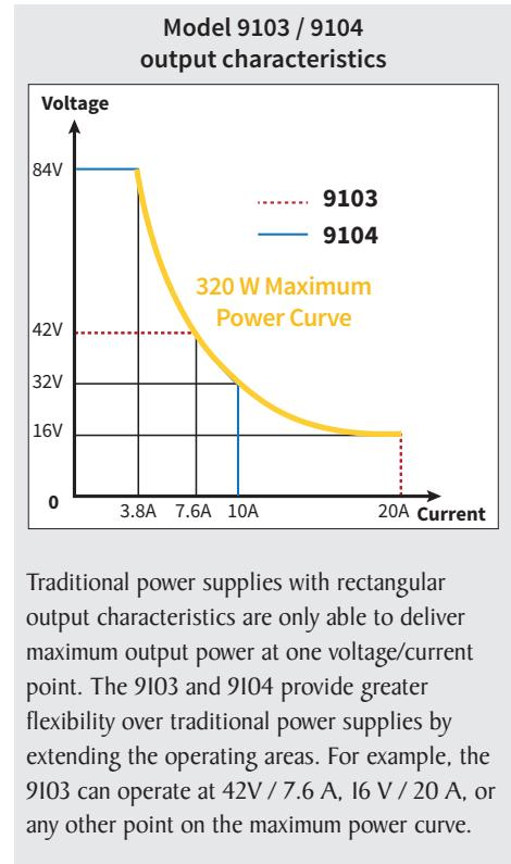
Traditional power supplies with rectangular output characteristics are only able to deliver maximum output power at one voltage/current point. The 9103 and 9104 provide greater flexibility over traditional power supplies by extending the operating areas. For example, the 9103 can operate at 42V / 7.6 A, 16 V / 20 A, or any other point on the maximum power curve.
