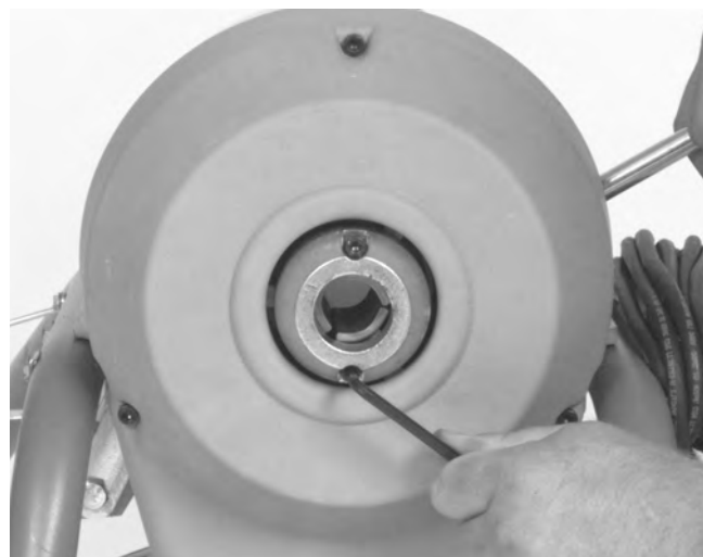
Figure 12 – Replacing Clutch Jaws
