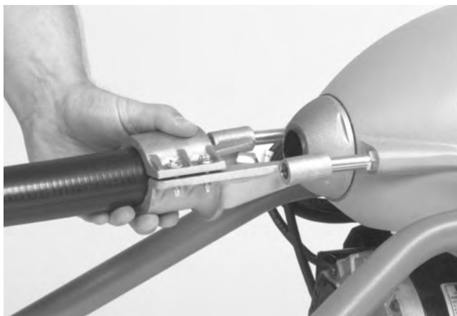
Figure 3 – Rear Guide Hose Attachment
