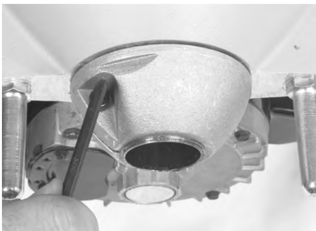
Figure 14 – Removing Clutch End Play
