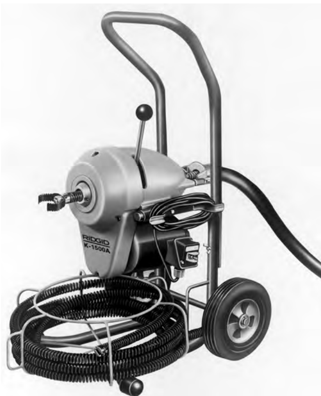
Figure 11 – Storing Cables On “A” Frame Models
