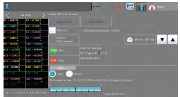
Comprehensive triggering capabilities: Configure triggers on analog and logic channels. Select from multiple combinations of thresholds, channels and conditions.
