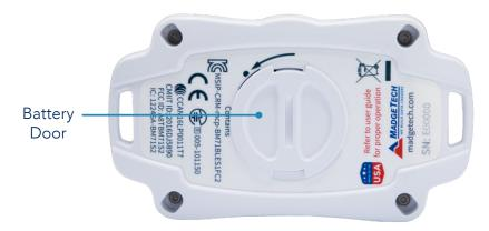
Either by pinching the finger impressions, or through using a coin, rotate the battery plug counter clockwise by 45 degrees. Remove the plug, and the battery becomes exposed.
