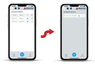
Ensure that Bluetooth is enabled on your smartphone, then press and hold the Bluetooth button on the LynxPro for 3-seconds until the Bluetooth logo appears in the upper left corner. When plugged into external power, Bluetooth will remain on.
