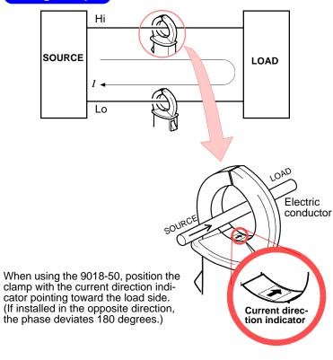
Attach the clamp around only one conductor. Single-phase (2wire) or three-phase (3-wire) cables clamped together will not produce any reading.
