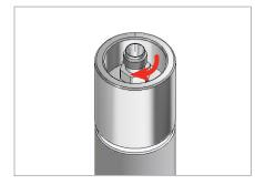
Screw the Fitting Body into the end of the stopper assembly (finger-tight).
