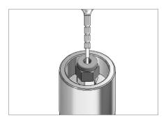
5. Feed the data logger probe throw the Compression Fitting until the base of the probe is tightly against the Dome Nut.
