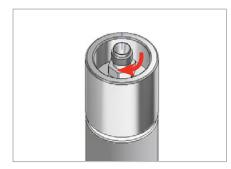
2. Screw the Fitting Body into the end of the stopper assembly (finger-tight).
