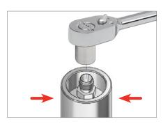
3. Holding the smooth metal end of the stopper, use a 7/16" wrench or socket to tighten the body into the stopper.
